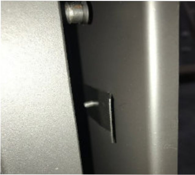
Tension clip on side of the body
