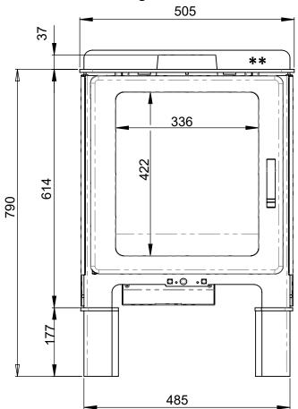
\*\* The additional, top flue rear convection panel (supplied loose within the stove) needs to be used when installing the stove 100mm from a combustible wall; this slots over the rear convection panel and provides additional radiant protection from the flue collar.
