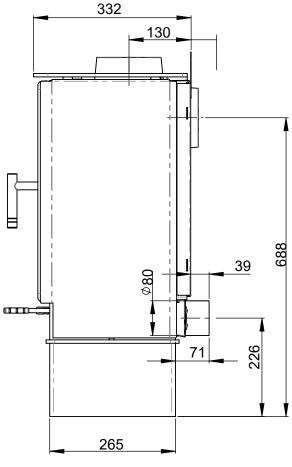
The direct air intake spigot (80mm diameter) to the rear of the stove is removable with a 2.5mm allen key.
