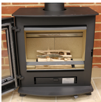
1. Put 2 small logs on a bed of ash spaced about 6-7cm apart. Place 1-2 firelighters in between and move air lever to right (fully open)
