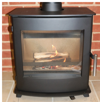
5. Place 2/3 logs on the hot embers and ensure that the wood is not stacked too closely with the air slider fully open. The wood will ignite in 2/3 minutes. Adjust the air slider for optimum combustion
