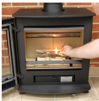
2. Neatly stack dry kindling on top of the logs in a # formation of approx 3 layers and light the bottom fire lighters
