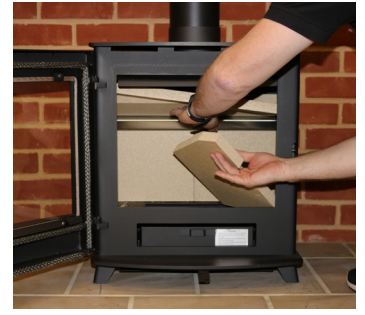
3. Ease the right hand side brick away whilst supporting the front baffle section with your other hand. Carefully manoeuvre both baffle brick sections out of the stove
