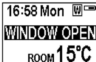
2b.45 After indoor temperature rise or manual intervention (by operating remote control), it will return to normal working state.
