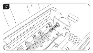
9.4 Withdraw the spindle from the left hand bracket, see Diagram 18. The spindle may need to be tilted to be removed from the location bracket.
