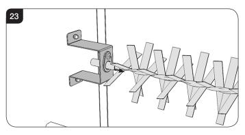
12.5 Replace in reverse order. Take care not to damage the spindle blades when replacing.
