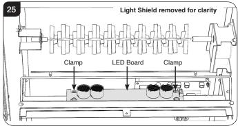
13.3 Push the rear clamp towards the rear of the firebox to release the board, see Diagram 26.
