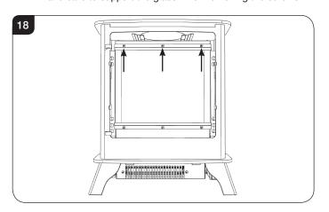
3.10 Carefully tip the glass forward and lift out of the bottom bracket to remove. Place carefully to one side.
