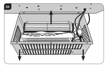
16.5 Disconnect the 4 coloured wires running from the firebox to the heater assembly, see Diagram 35 noting the orientation.
