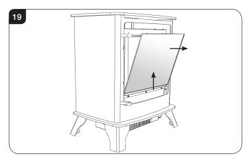
Note: When refitting the glass ensure that the top and bottom glass seals are in position on the glass. The bottom seal may remain in the bottom bracket, if this occurs it will be necessary to carefully extract the seal and centrally reposition on the bottom of the glass before reinstalling.
