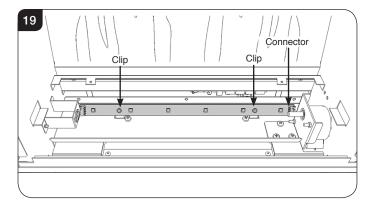
10.4 Fitting a new board is the reverse of this process.
