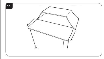
5.6 Make sure the appliance top fits into the guide along the bottom of the canopy, see Diagram 12.
