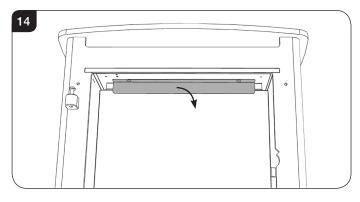
8.2 Supporting the glass, carefully tilt the appliance forward slightly and lower the top of the glass, see Diagram 15.
