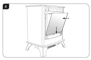
5.2 Raise the top of the glass and secure with the bracket and 3 screws, see Diagram 9.
