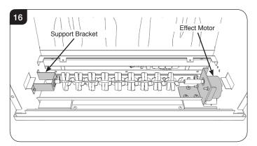
9.3 The Effect Spindle is attached to the Effect Motor by a rubber sleeve.Pull the rubber sleeve off the Effect Motor axle, see Diagram 17.
