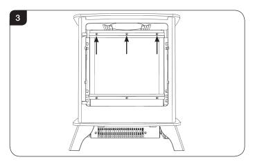
3.7 Carefully tip the glass forward and lift out of the bottom bracket to remove. Place carefully to one side.
