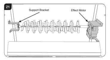
12.3 The Effect Spindle is attached to the Effect Motor by a rubber sleeve.Pull the rubber sleeve off the Effect Motor axle, see Diagram 22.
