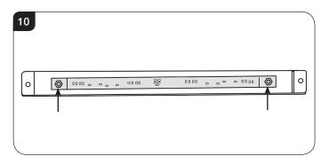
5.5 Disconnect the wire from the LED board.
