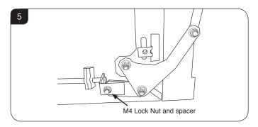
Withdraw the burner unit from its location.
