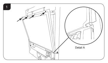
1.7 The glass frame must be refitted to the appliance following cleaning or servicing.
