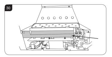
6.25 Remove the front channel from the top of the burner unit by undoing the 2 screws, see Diagram 31.
