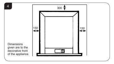
2.8 The maximum depth of combustible shelf is 150mm at a minimum height of 300mm above the decorative front.
