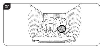
6.16 Place a second single large coal in the middle dent of the front coal resting against the flame baffle, see Diagram 28.
