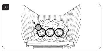
6.19 Place two of the remaining small coals in the spaces next to the first. The final small coal sits at the front right next to the large coals, see Diagram 31.
