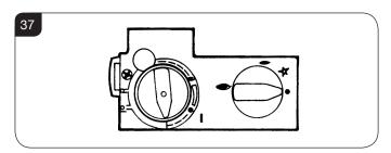
8.9 Press in the right-hand control knob and rotate anticlockwise until a click is heard. Continue to press in. The knob points to the pilot (—).
