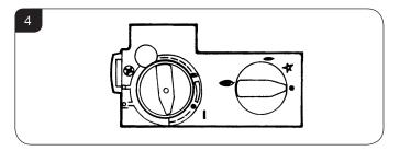
2.9 Press in the right-hand control knob and rotate anti-clockwise until a click is heard. Continue to press in. The knob points to the pilot (—).
