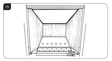
5.12 Position the flame baffle centrally on the tray and ensure the stepped lower edge engages against the rear edge of the burner skin, see Diagram 16.
