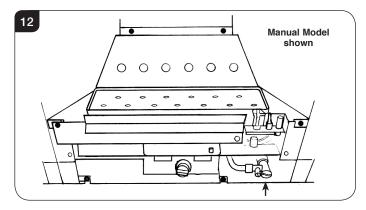
4.13 Carefully refit the burner assembly.
