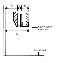
The appliance can also be fitted into a metal flue box with a 5" (125mm) diameter flexible liner. In this installation a 1" (25mm) rebated fire surround must be used. Refer to Diagram 2 for dimensions.
