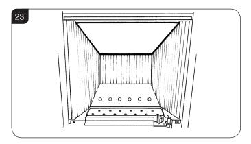
6.12 Position the flame baffle centrally on the tray and ensure the stepped lower edge engages against the rear edge of the burner skin, see Diagram 24.
