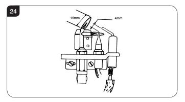
5.14 After reassembly check for gas soundness and carry out a flame failure functional check as detailed in the Fault Finding chart, especially the time it takes for the mag unit to close.
