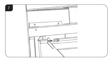
1.22 Carefully remove the enamel back panel by rotating it out of the firebox.
