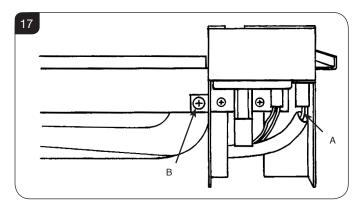
5.2 Lift the shroud up and away from the pilot unit.
