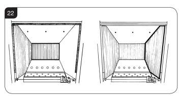
6.10 Locate the top panel on top of the sides and rear by lifting it up and forward inside the box. 6.11 Slide it backwards and down behind the side panels to rest on the rear panel, see Diagram 23.
