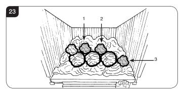
5.20 Finally position the Half Moon coal on the top right as shown, see Diagram 24.
