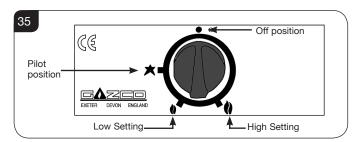
YELLOW FLAMES APPEAR WHEN THE APPLIANCE HAS REACHED SUFFICIENT HEAT – (10 TO 20 MINUTES). IF THE APPLIANCE IS EXTINGUISHED OR GOES OUT IN USE, WAIT 3 MINUTES BEFORE TRYING TO RELIGHT.
