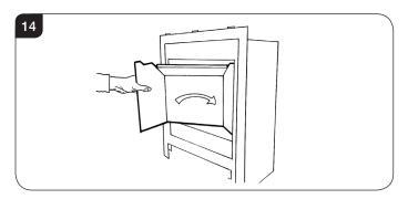
5.2 Check that the panel is sitting behind the rear ledge of the burner, see Diagram 15.
