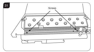
6.26 Undo the 2 screws securing the bracket to the bottom of the burner unit, see Diagram 21.
