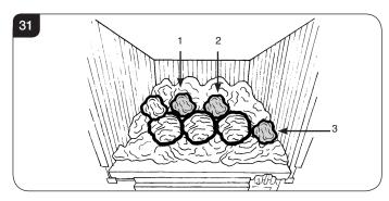
6.20 Finally position the Half Moon coal on the top right as shown, see Diagram 32.
