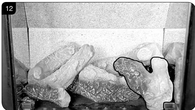
7.7 Place the pointed bottom of log D into the corner of the burner tray and rest on the location stud in log B, see Diagram 12.
