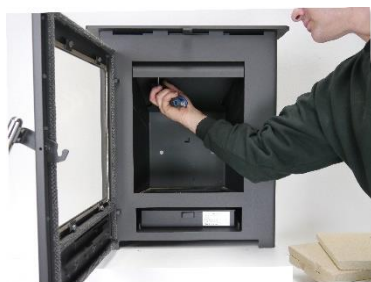
1. Two M8 allen key bolts holds the upper steel baffle in place. Undo by 1-2 turns
