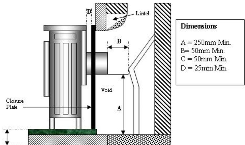
Before you install the stove, make sure the chimney flue outlet is correctly positioned to align with the flue outlet on the stove and that the chimney is in good condition. If not, a chimney liner must be installed or a suitable class II gas flue used. A draught is necessary to ensure the products of combustion are fully evacuated.
