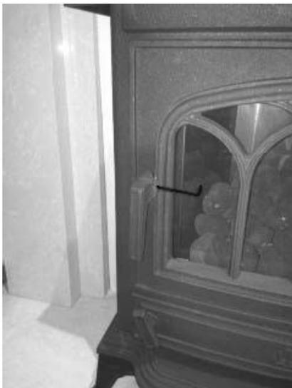
2. Slide the door handle over the hex nut ensuring that the handle is in the downwards position. Using the Allen key and grub screw (supplied) secure the handle in position.
