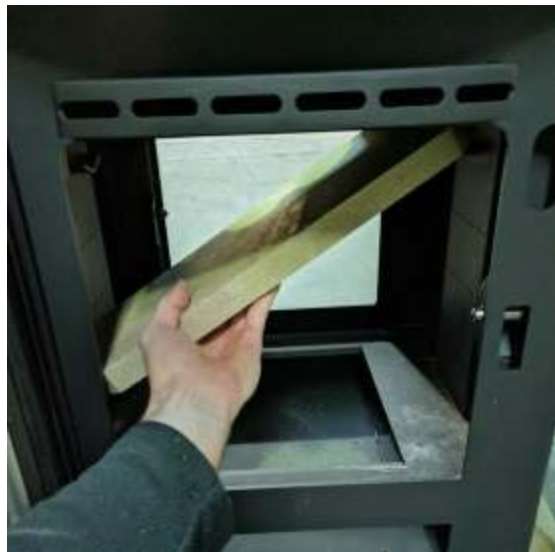
6: Manoeuvre the Baffle Brick off the support brackets and then angle the brick in order to extract it from the combustion chamber.
