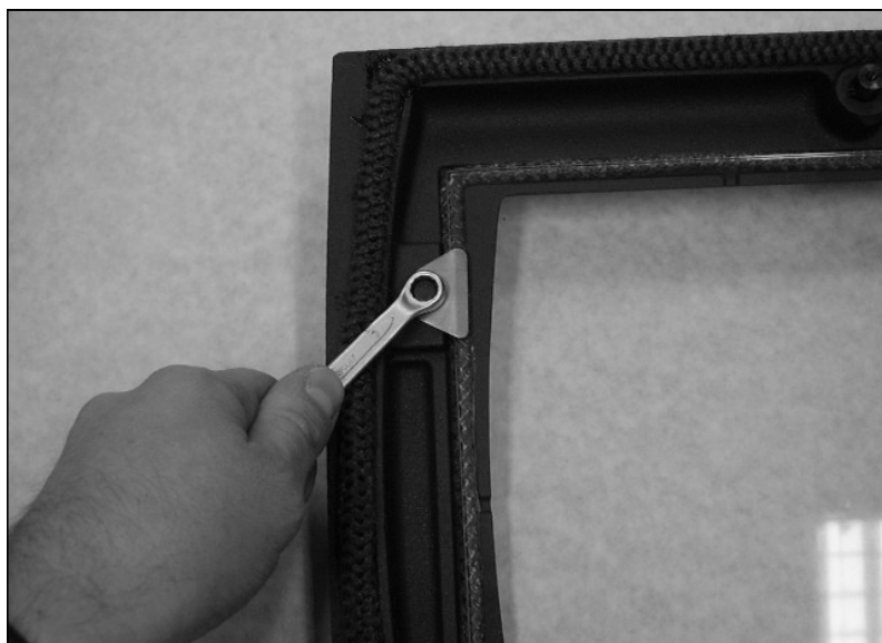
Fig. 11. Tightening The Glass Clip
