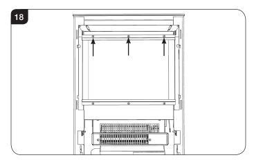
3.9 Carefully tip the glass forward and lift out of the bottom bracket to remove. Place carefully to one side.
