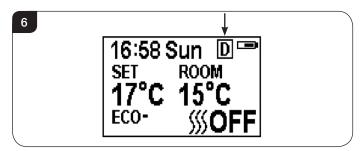
2b.11 Hold the → button for 6 seconds to enter the daily heating setting.
