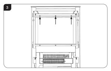
3.5 Carefully tip the glass forward and lift out of the bottom bracket to remove. Place carefully to one side.
