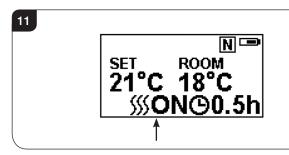
Note: It is normal for the fan heater to stop running for periods of time. This happens if the room temperature is higher than the temperature set on the control.
